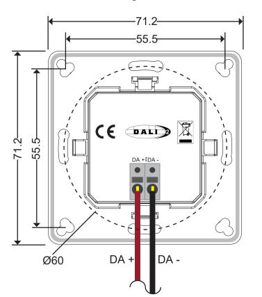
Fitted Panel side view (Measurements are in mm)
