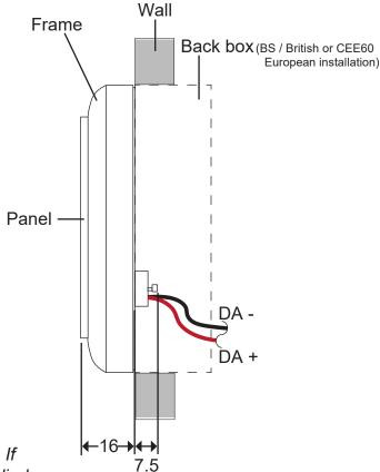
Note: Only one cable per terminal pole allowed. If looping is required then use the terminals supplied with the panel or other suitable terminals.
