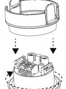
Place the circular insert onto the sensor and lock into place by rotating until fully secured.
