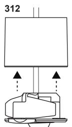
Note: Take care when placing the sensor into the mounting box. Ensure the fully fitted sensor sits secure and flush to the mounting box edge and no gaps are present.
