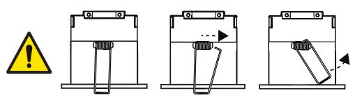
Ensure the two side springs are repositioned so they sit on the rim of the unit and are not an obstuction when fitting the sensor into the mounting box.
