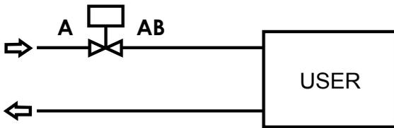
b) Constant flow when used in injection circuits
