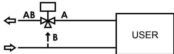
d) Constant flow mixing when used in injection or tapping circuits
