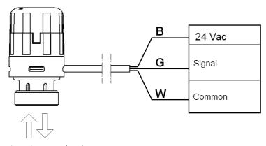
B = brown (24 V AC - 50/60 Hz) G = green (control signal 0-10 V DC)W = white (common)
